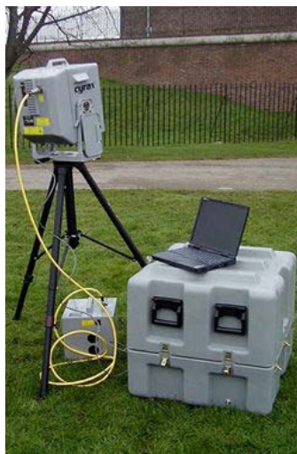
Figure 9 Laser Scanning Equipment (CyraX 2500)
